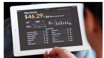
Figure 1: Example real-time interface of electricity usage and appliance-level breakdown in the home using the ElectriSense technology. Video Figure Link
