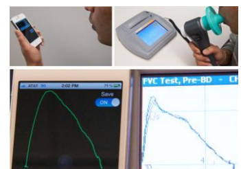
Figure 7: SpiroSmart (left) measures lung function (spirometry) using the mobile phone's built-in microphone and produces accurate results similar to a traditional clinical spirometer (right).
